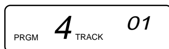
Select track number directly or with the SKIP button. Press PROGRAM to store
