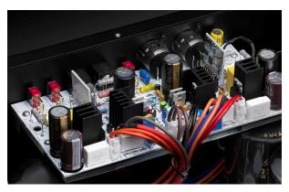
The JC 1 driver stage was an excellent single-stage circuit. Curl predicted that a two-stage cascode driver would make a substantial performance improvement because a driver circuit with cascode topology has some of the favorable attributes of vacuum tubes, namely higher input-output isolation, higher input impedance and higher output impedance. Its greater bandwidth and open loop gain were expected to improve linearity and a noticeable improvement in sound quality. This proved to be true.
