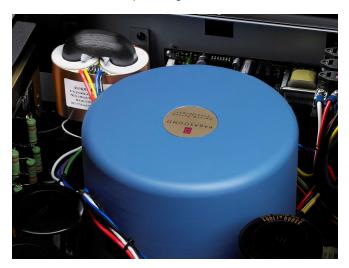
Supporting this substantial current required an even more potent power transformer. The massive 2.1 kVA transformer weighs 30 lb. (13.6 kg) - 30% more than its predecessor. Developing this power transformer was challenging and required 11 hand-made samples before we achieved the necessary power and total absence of mechanical vibration. The JC 1+ power transformer accomplished this with an especially potent and expensive steel core.
