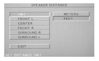
Use a measuring tape and note the distance from your primary listening position to each speaker. The D 3 will translate each foot (.34 meters) of distance for a given channel into 1ms (millisecond) of delay. For each speaker, the distance can be set in 1-foot increments from 5 to 30 feet (or 1.5 to 9 meters, if you set the UNITS for METERS).
